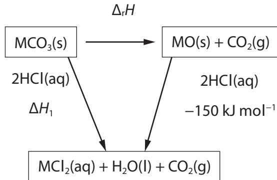
In an experiment to determine  $\Delta H_1$ , 0.050 mol of  $\text{MCO}_3$  was placed in a  $100 \text{ cm}^3$  beaker.  $60 \text{ cm}^3$  of  $2 \text{ mol dm}^{-3}$  hydrochloric acid (an excess) was added and the mixture stirred. The maximum temperature rise measured was  $6.0^\circ\text{C}$ .
